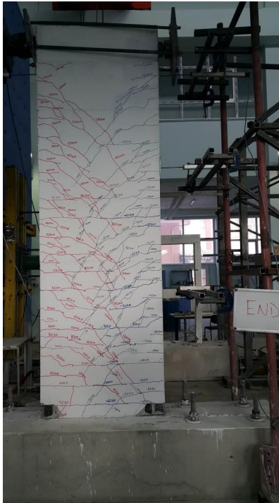
Figure 11. The final crack distribution of the experimental specimen at the end of the loading procedures.
